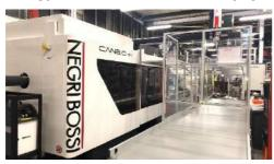
Melting and injecting plastic at high temperatures and pressures requires a lot of energy, moulding machines manufactured in the 1990's typically using one whole kilowatt of power to process just a kilo of raw material!
