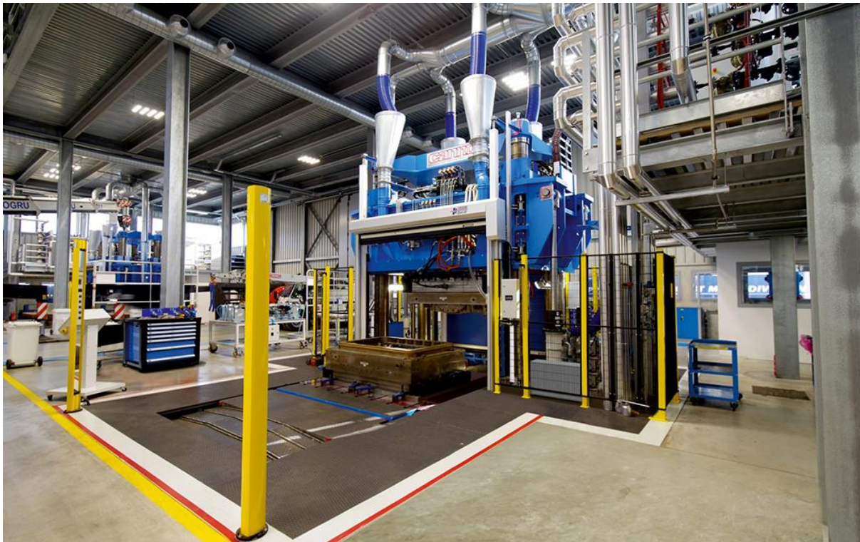
Figure 1 - A CANNON short-stroke press, similar to the machine TEP has ordered
