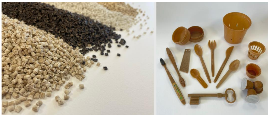
Figure 2 Solinatra material grades (left) and a variety of products moulded from Solinatra’s material (right)
